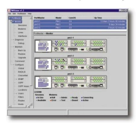
Backing up configurations is equally straightforward. You can save the entire configuration of a device to a file, or select just one or more subsystems. All backups are written as ComOS CLI text, so you can read or edit the file using a simple text reader. Command files can also be restored to a PortMaster, and the complete restoration, including ComOS responses, can be logged to a file.
